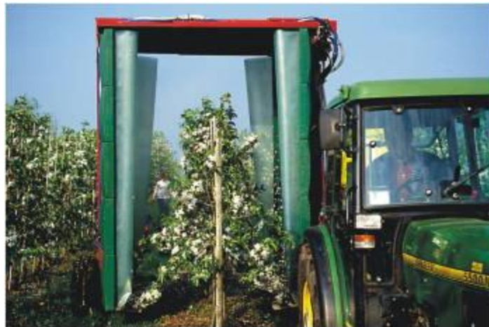
Figure 1.7. Tunnel sprayer ( www.lipco.com )
