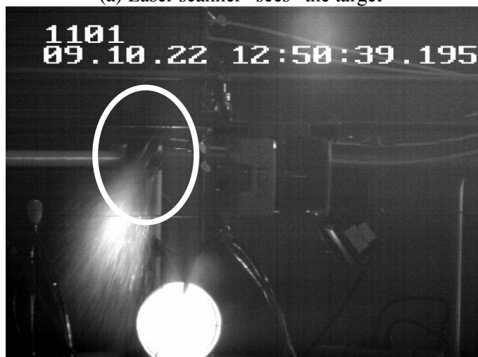
(c) Full spray discharged from nozzles
