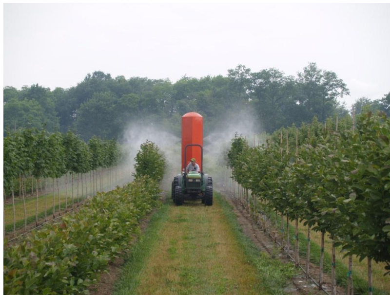
Figure 1.3. Overspray of a nursery sprayer when using the same setting to treat different size crops in the same production line
