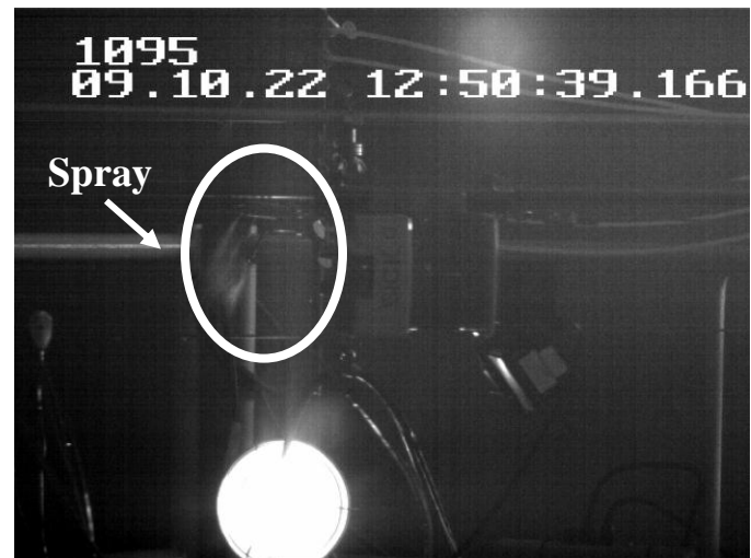
(b) Nozzles start spraying
