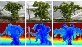
LiDAR mapping of individual trees. Blue areas identify spray target and volume based on foliage density.
